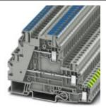
Ground modular terminal block, Connection method: Screw connection, Cross section: 0.14 mm² - 6 mm², AWG: 26 - 10, Width: 6.2 mm, Height: 60.1 mm, Color: gray, Mounting type: NS 35/7,5, NS 35/15
